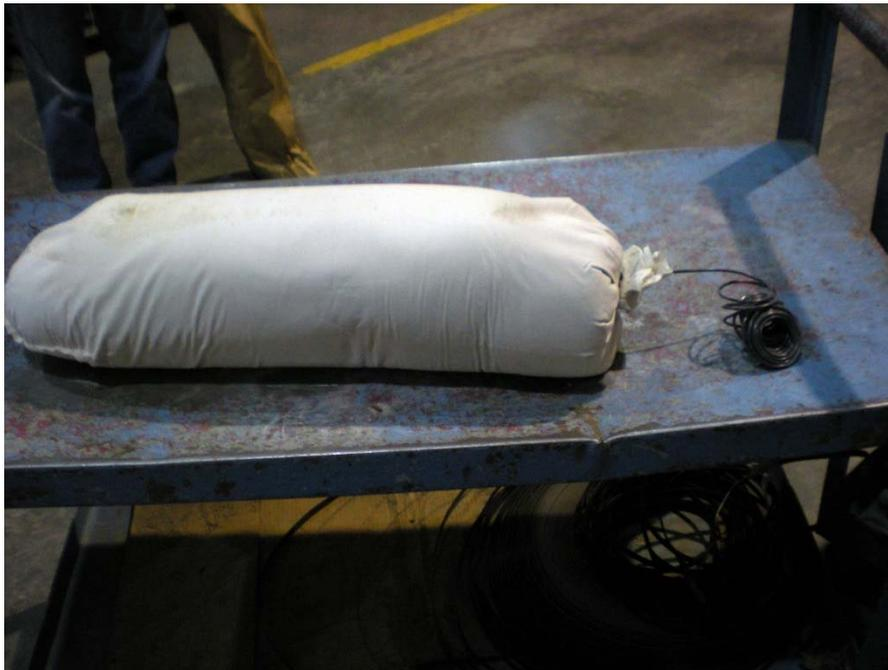
Figure 4 – Prepackaged Sacrificial Anode
